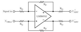
Figure 3: Schematic of the DC-coupled analog input circuit. For each channel U<sub>Offset</sub> can be set by 16-bit DACs.
