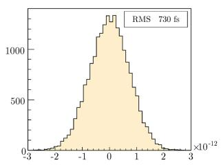
Figure 4: Time interval error of the sampling clock.
