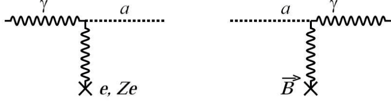
Figure 3.1: The Primakoff effect in the Sun: a photon converts into an axion in the presence of fluctuating electric fields (left). In a laboratory magnetic field the inverse process can take place and an incoming solar axion can couple to a virtual photon provided by the transverse magnetic field resulting in a real photon (right). Image taken from Ref. [3].
