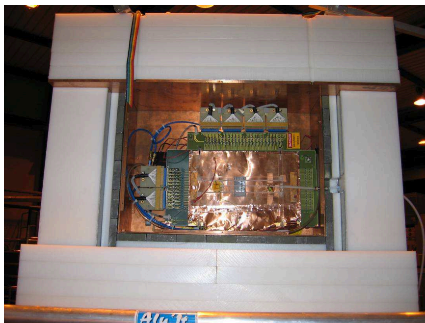
Figure 4.7: TPC with shielding added before data taking runs in 2004 [100]. It is possible to see all layers of the shielding (copper box, lead, cadmium and polyethylene).
