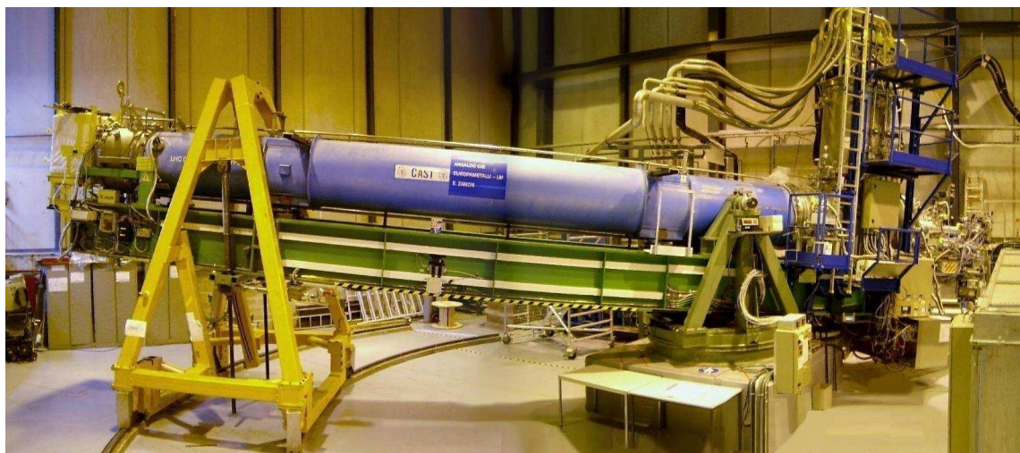
Figure 4.2: The CERN Axion Solar Telescope in the experimental area. The magnet (blue) is borne on a platform (green), which is supported on the right hand side by a turntable (olive green) allowing horizontal movement, while it is carried by two screws at a girder (yellow) for enabling vertical movement on the other end (left in image) [94].
