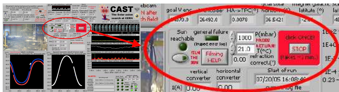
Figure 4.17: Filming software implemented in the tracking program (User Interface on tracking PC). If the Sun is within the range of movement of the magnet, a green light can be seen. Any occurring error will show up by a light as general failure. In order to activate the Filming Mode of the software, the “Film the Sun” button has to be pushed. The Filming Help button provides additional information on pressure and temperature, which have to be entered. If done so, the refraction correction is displayed and logged as well.
